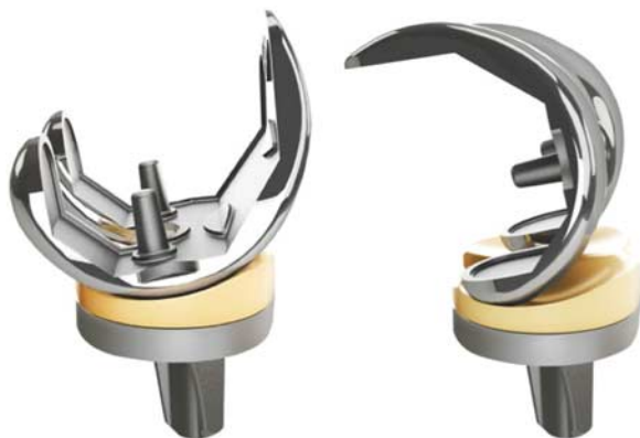
FIGURE 1. The anterior cruciate ligament-substituting total knee arthroplasty design incorporates a lateral tibiofemoral compartment that is spherically conforming in extension, which becomes progressively more lax in flexion to allow the condyle to translate posteriorly. full color online
